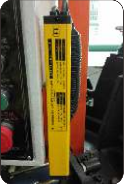
Light Scanner Safeguard safety for worker
